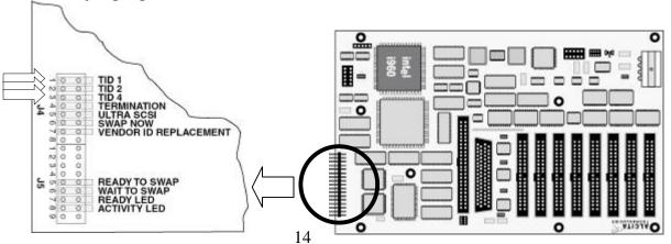
The first three jumper pairs control the SCSI-ID selection for the host SCSI interface. When the jumper is present, this pin pair is CLOSED. The three pairs can be jumped or connected to a rotary SCSI-ID selection switch on the rear of the storage enclosure. The output of any selection switch must be routed to the open/closed signal pins on the top of each pair and the bottom pins, closest to the circuit board, connected to the common leg of the switch.
