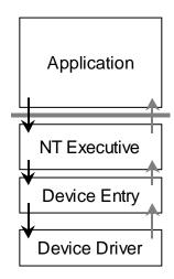
Figure 1, Composition of a Kernel-Mode Driver.
