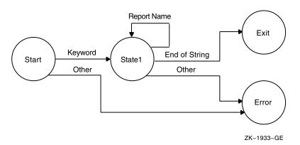
Another technique for developing a state table starts with a tabular diagram in which the first column is the starting state, the second column identifies the input token, or keyword, and the third gives the resultant state.
