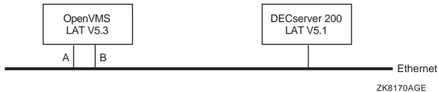
When a LAT connection is started between the DECserver 200 and the OpenVMS system, the LAT software determines that it is possible to use both adapters A and B for the LAT virtual circuit. One of the adapters will be chosen as the primary communications path while the other will be present in the unlikely event that the primary path fails.
