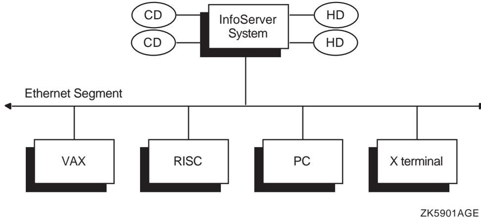
You can connect the InfoServer system to your Ethernet LAN and turn on the system. After the server is initialized, or **bootstrapped**, the server software automatically serves to client systems the device media connected to it. If you insert a compact disc into a server drive, the server detects this new device and automatically serves it to client systems by using the volume label as the service name.
