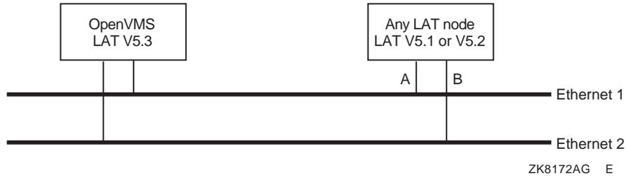
Any configuration similar to this diagram will result in unpredictable results and may not function. In a network environment, LAT Version 5.1 and 5.2 nodes can have only a single logical LAN address. The configuration in Figure 12-5 violates this rule. The configuration shown in Figure 12-4 is a valid alternative.
