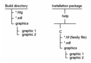
Figure 13-2 Relationship of build directories and installation package
