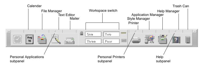
Figure 1-1 Front Panel controls
