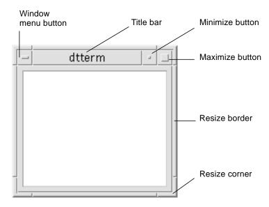
Figure 1-2 Window frame controls
